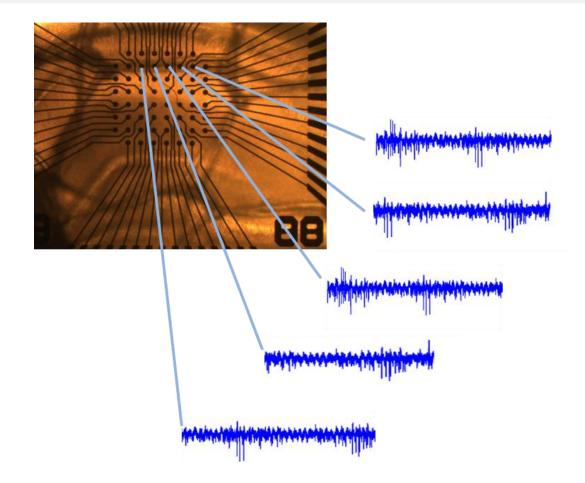
Within each tested slice, the CA1 neurons spontaneous activity is recorded at 3 to 8 electrodes, each electrodes recording the activity of several neurons located in the vicinity. The results obtained are averaged from a large number of neurons and are then very robust. Several concentrations of a compound could also be evaluated on a single slice.
