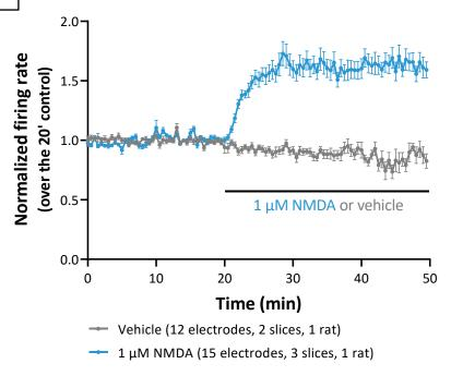
NMDA bath applied onto the hippocampal slices strongly increased the firing rate of CA1 pyramidal neurons.
